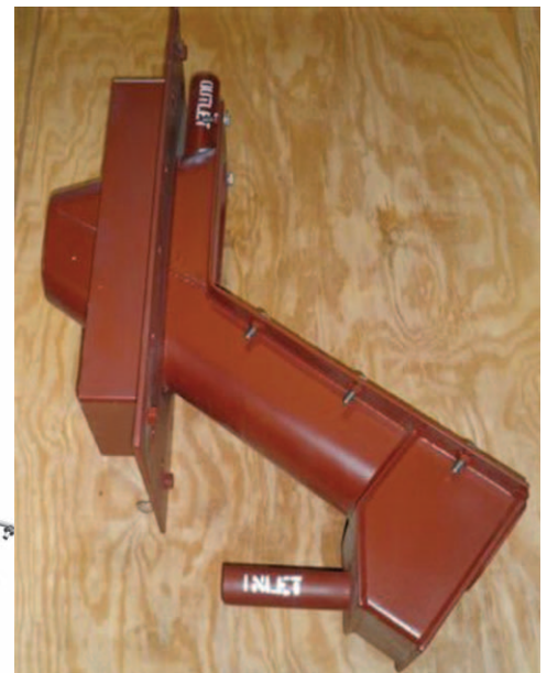
Smelt Spout with Refractory Seal Box
