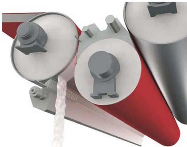
Figure 2. SingleForce provides proven automated and ropeless tail threading in single-felted dryer groups.
