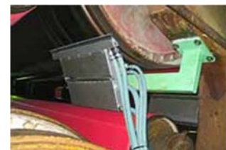
Figure 14. Valmet Tail Threading Double Fabric tail threading units thread the tail through the PM2 LWC line by means of compressed air.
