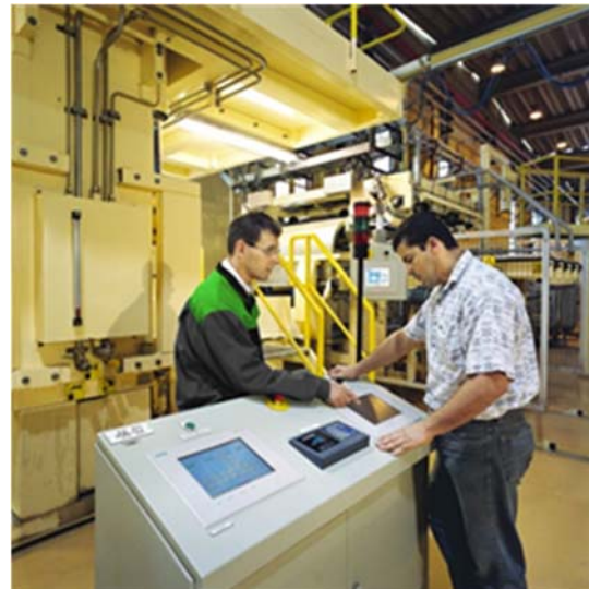
Figure 13. A modern HMI will greatly reduce the complexity of a machine control benchboard, making it easier to operate (and maintain).
