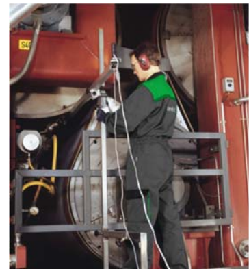
Figure 6. Highly trained experts will collect data onsite before producing their analytical report. In this case dryer surface point measurement is occurring.
