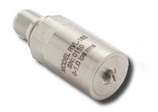
RVL-165 is a true RMS velocity output sensor for mechanical condition monitoring. It is typically used for continuous overall vibration level monitoring in industrial control systems. The sensor provides a 4-20 mA output and can therefore be easily connected to any PLC or DCS.
