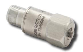
RVT/TT-125 is an industrial accelerometer with internal temperature sensor. Dual output sensor is an optimal solution for condition monitoring applications that utilize both vibration and temperature measurements.
