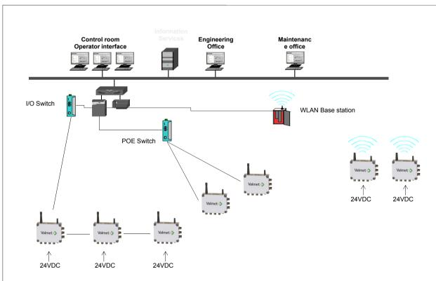
Connection possibilities into Valmet DNA Machine Monitoring
