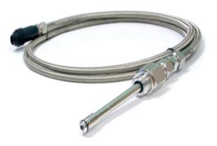
RPT-122 is a sensor for measuring dynamic pressure variations in process. It is typically used for monitoring pulsations in paper machine short circulation and head box, and pneumatic pulsations in doctor blade loading devices. Synchronized measurements can be
